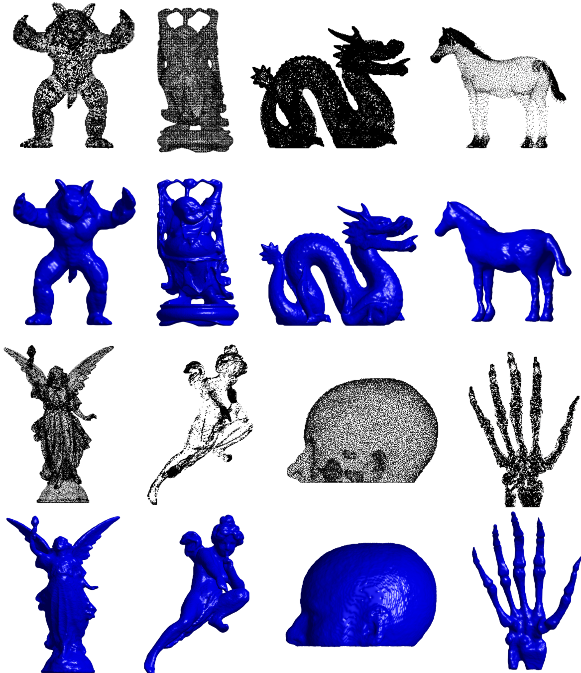
Figure 5.11: Surface reconstruction from point clouds using the proposed method. 1st and 3rd rows: point clouds; 2nd and 4th rows: reconstructed results.
